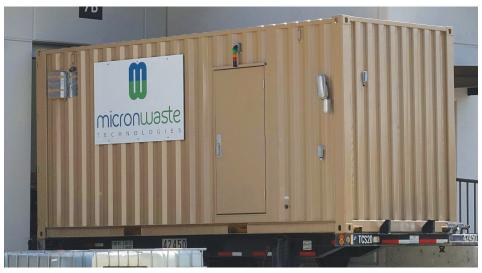
Vancouver-based Micron Waste's Cannavore cannabis waste digester technology was patented in 2019. The first-of-its-kind system pulverizes cannabis waste material in combination with microbes and enzymes to compost material and fits in a regular shipping container for transport.
